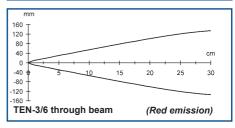
The operating distances indicate the detection distance with standard fibre-optics (refer to **OF** series) and excess gain 2.
